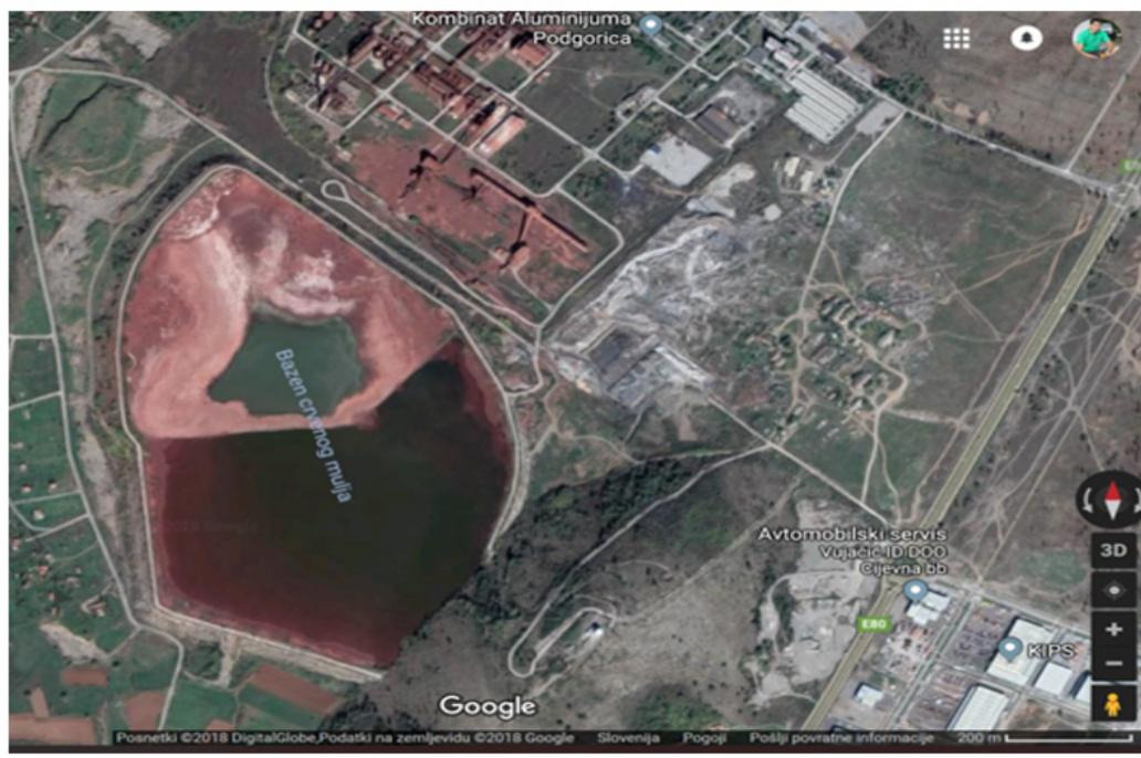
Figure 1: Aerial view of the tailing of red mud near Podgorica.
