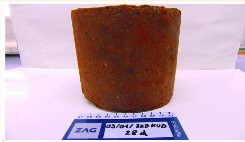
Figure 9: Geotechnical composite made of red mud and paper ash (courtesy: P. Oprčkal).
