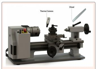
**Figure 3:** Thermal data acquisition system using infrared thermometer. Adapted from [11].
