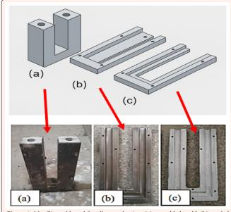
**Figure 1:** Metallic mold used for alloy production: (a) assembled mold, (b) sanded surface, and (c) mold coated with kaolin.
