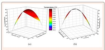
**Figure 5:** 3D surface plots of cutting temperature: (a) as a function of cutting speed and diameter; (b) as a function of cutting speed and time.
