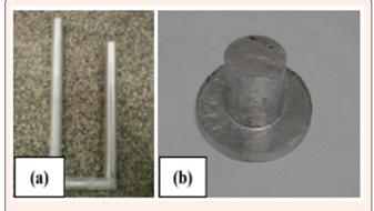
Figure 2: (a) Cast U-shaped ingot and (b) sample for chemical analysis.
