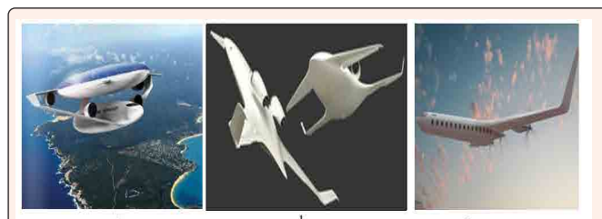
Figure 3: New WB Aircraft Concepts: a- Criplane Disc Body with LH 2, b- Canard WB Version and c- T-WB Hybrid E-Aircraft.
