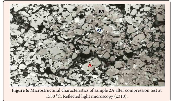
Figure 6: Microstructural characteristics of sample 2A after compression test at 1550 °C. Reflected light microscopy (x310).
