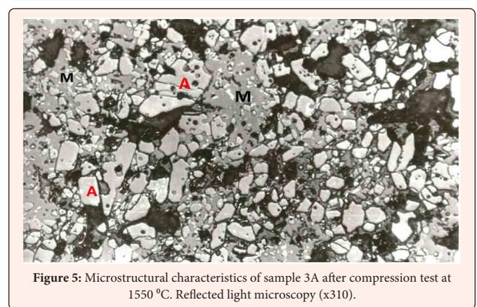
Figure 5: Microstructural characteristics of sample 3A after compression test at 1550 °C. Reflected light microscopy (x310).
