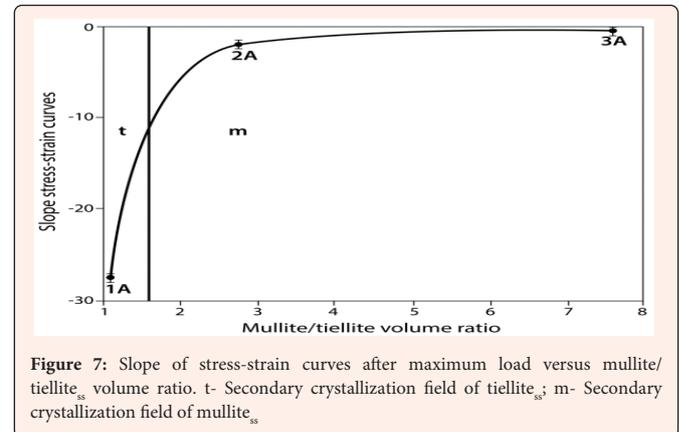
Figure 7: Slope of stress-strain curves after maximum load versus mullite/tiellite<sub>ss</sub> volume ratio. t- Secondary crystallization field of tiellite<sub>ss</sub>; m- Secondary crystallization field of mullite<sub>ss</sub>
