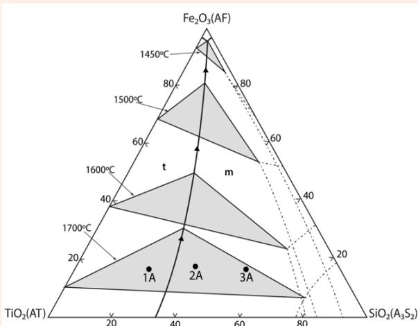
**Figure 1:** The  $Al_2O_3$ - $SiO_2$ - $TiO_2$ -Iron oxide quaternary system in air. Location of synthetic refractory bauxites on the projection (86 wt. %  $Al_2O_3$  plane) of the primary volume of alumina and tie-tetrahedroms at 1450°, 1500°, 1600° and 1700 °C where alumina<sub>ss</sub>-mullite<sub>ss</sub>-tiellite<sub>ss</sub> and liquid phase coexists in equilibria at indicated temperature. Tie-tetrahedroms determine the temperature of liquid formation, 1700° for studied sample.
