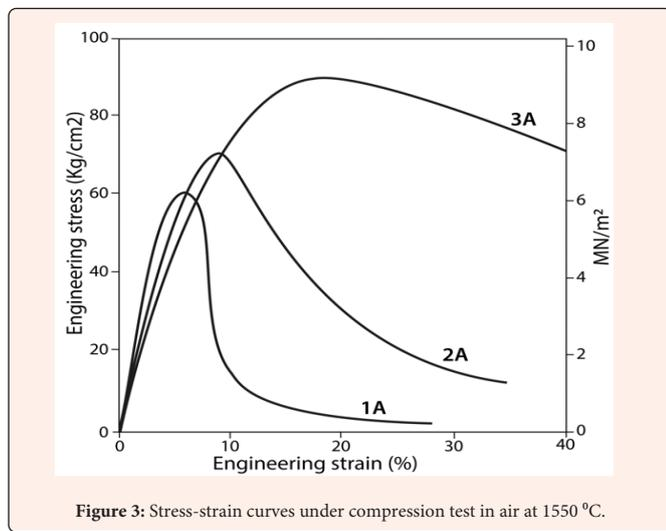
Figure 3: Stress-strain curves under compression test in air at 1550 °C.
