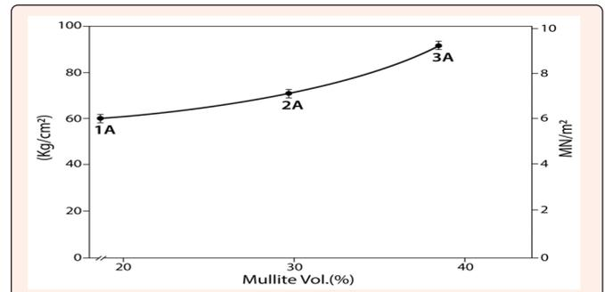
Figure 4: Maximum load supported by samples versus mullite vol.% content.
