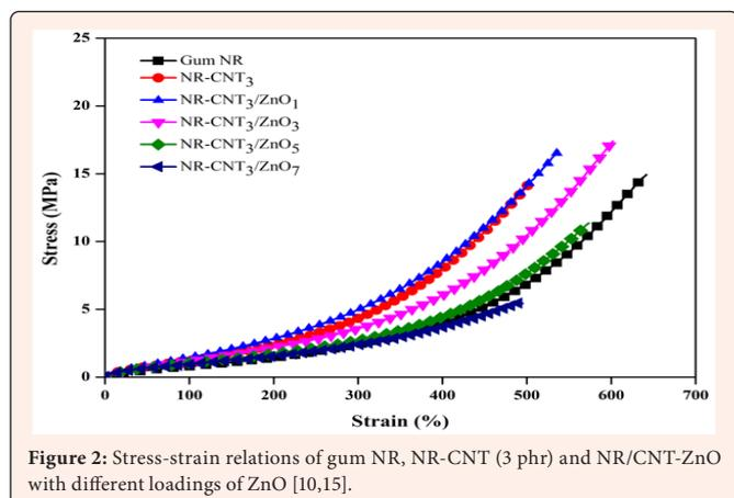
Figure 2: Stress-strain relations of gum NR, NR-CNT (3 phr) and NR/CNT-ZnO with different loadings of ZnO [10,15].
