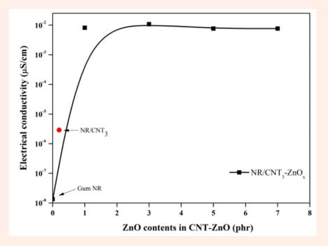
$Figure 1: Electrical \ conductivity \ of \ gum \ NR, \ NR-CNT \ (3 \ phr) \ and \ NR/CNT-ZnO \ with \ different \ loadings \ of \ ZnO \ [10,15].$
