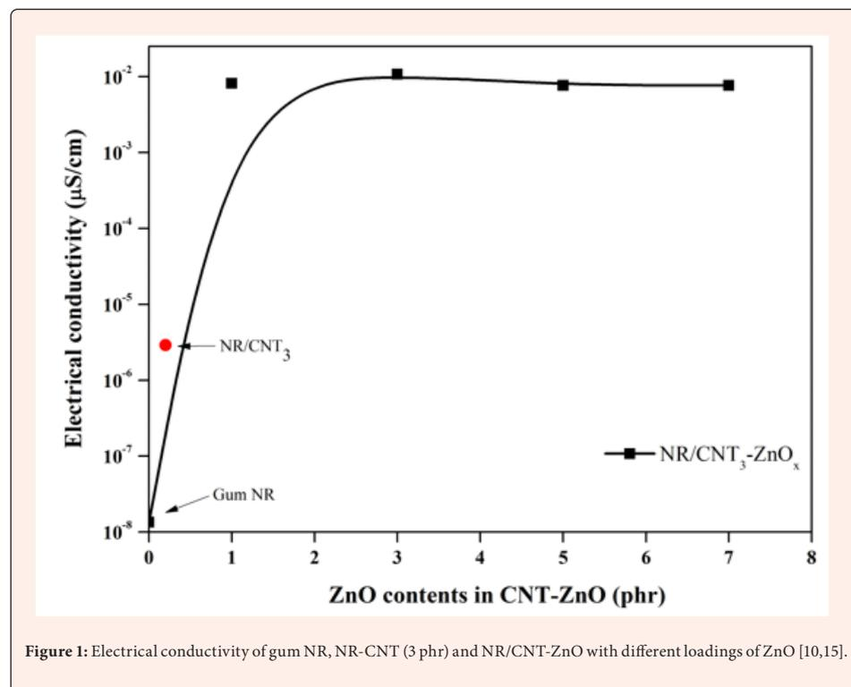
Figure 1: Electrical conductivity of gum NR, NR-CNT (3 phr) and NR/CNT-ZnO with different loadings of ZnO [10,15].
