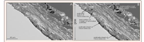
Figures 1A & 1B: Illustration showing features of 1. laminated patina with an invading leading edge of a micro-breccia patinelle, 2. the former surface of the glass as a straight, sharp edge (arrowed), and 3. thin sheet of supra-patina crust composed of (a) massive (structureless) silica, (b) silt- and dust-sized mineral particles, and (c) micro-vughs or 'caverns'.
