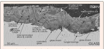
**Figure 3:** Crust of patina on glass showing a selected range of microstructures; prominent here is the corroded contact between patina and glass, colloform structures, the inter-lamination of silica (medium grey) and calcite (light grey), and layer-parallel desiccation cracks (thin black lines).
