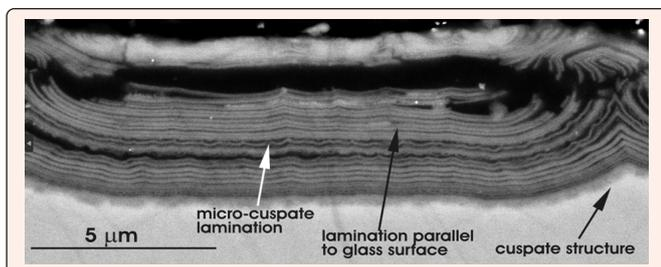
**Figure 4:** Largely parallel laminated patina, with thin layer of smaller-scale micro-cusate structures.
