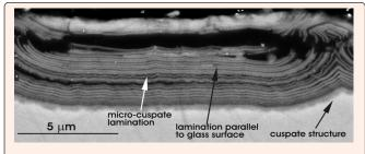
Figure 4: Largely parallel laminated patina, with thin layer of smaller-scale microcuspate structures.
