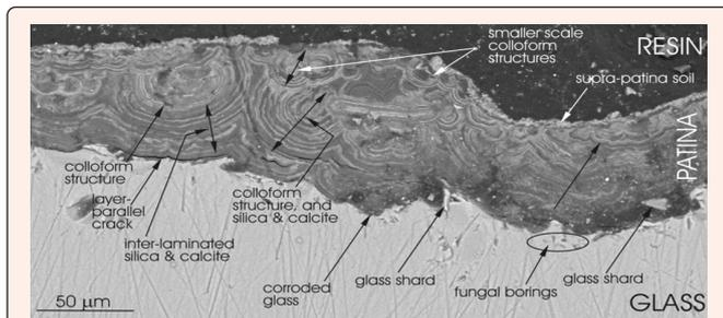
**Figure 3:** Crust of patina on glass showing a selected range of microstructures; prominent here is the corroded contact between patina and glass, colloform structures, the inter-lamination of silica (medium grey) and calcite (light grey), and layer-parallel desiccation cracks (thin black lines).
