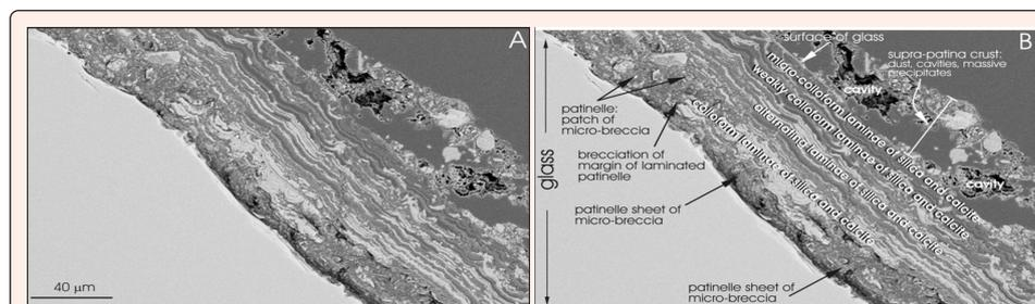
**Figures 1A & 1B:** Illustration showing features of 1. laminated patina with an invading leading edge of a micro-breccia patinelle, 2. the former surface of the glass as a straight, sharp edge (arrowed), and 3. thin sheet of supra-patina crust composed of (a) massive (structureless) silica, (b) silt- and dust-sized mineral particles and (c) micro-vughs or 'caverns'.
