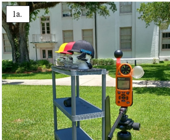
Figure 1a: Orientation of the cricket helmets to radiant heat characteristic of 1035 hr CST and environmental monitoring system used during measurements of mean ( \pm SD) helmet shell cover temperature, T_{hsc} (°C).
