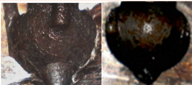
Figure 3: Sac volume of the old nozzle and the new nozzle.
