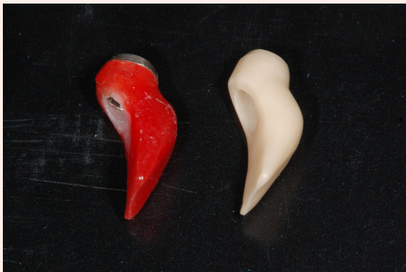
Figure 10: Abutment produced through MAD/MAN processing: resin mock-up (left) and milled zirconia abutment (right).
